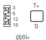
Long-time delay time setting dials, customer use proper tools for 4 specific settings (3-18)s of overcurrent at  $6x\ensuremath{\mbox{R}}$
