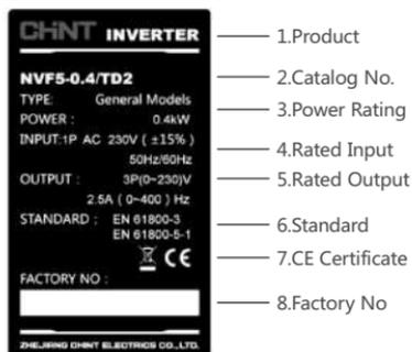
Figure 2-1 Nameplate of NVF5 series inverter
