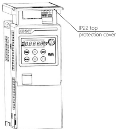
Figure 7-2 Product outline after installing IP22 protection cover
