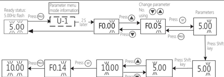
Figure 7-12 Parameter setup in Simple menu mode
