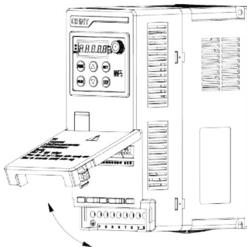
Figure 7-4 Cover usage of NVF5-3.7/TS4-B~NVF5-7.5/TS4-B
