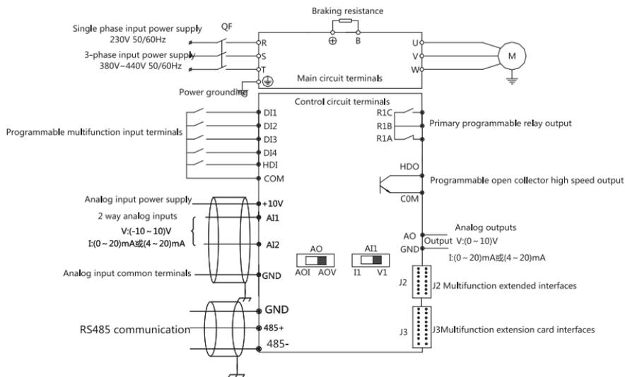
Figure 5-3 Wiring diagram of NVF5-0.4TD2~NVF5-7.5/TS4 terminals
