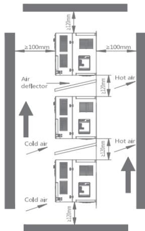
Figure 3-2 Vertical installation of multiple inverters
