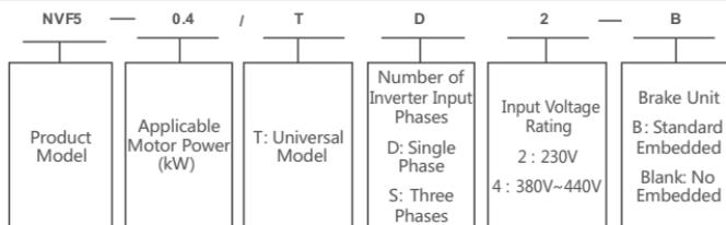
Figure 2-3 NVF5 series inverter type key definitions
