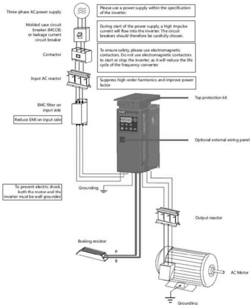
Figure 7-7 Peripheral components of main circuit
