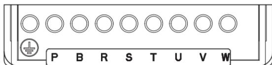
Figure 5-5 Main circuit terminals NVF5-0.4/TS4-B~7.5/TS4-B
