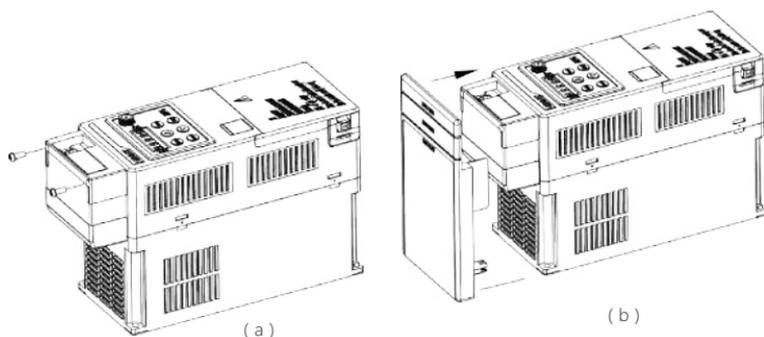
Figure 7-1 Installation diagram of IP22 protection kit
