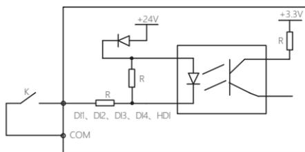
**Figure 5-7 Connection method using internal +24V power**
