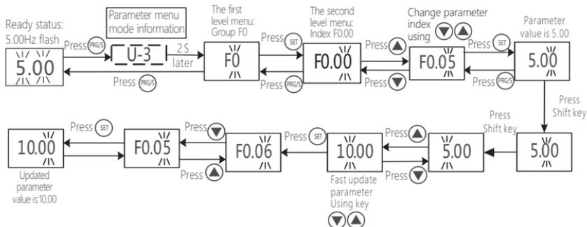
Figure 7-15 Parameter setup in Engineering menu mode
