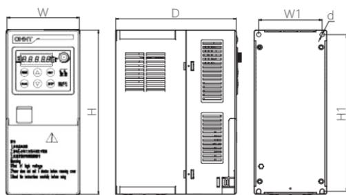
Figure 6-2 Outline and installation dimensional drawing of NVF5-3.7/TS4-B~NVF5-7.5/TS4-B,
