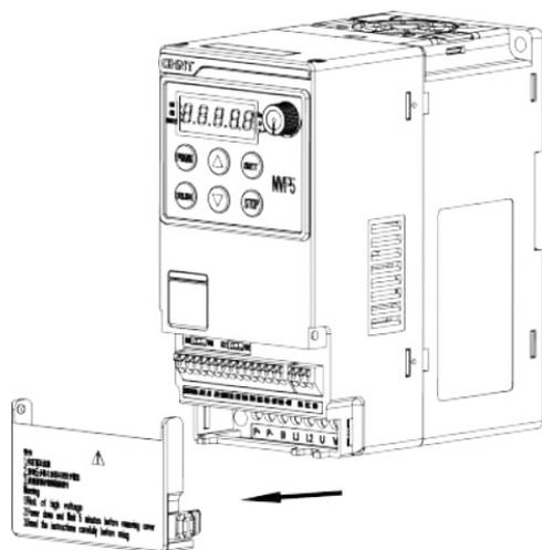
Figure 7-3 Cover usage of NVF5-0.4/TD2~NVF5-2.2/TS4-B,
