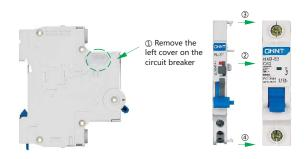
After AL-X1 is assembled with the circuit breaker, mount them on the TH3.5-7.5 steel mounting rail.
